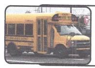
A Type "A" school bus is a van conversion or bus constructed utilizing a cutaway front-section vehicle with a left side driver's door. The entrance door is behind the front wheels. The definition includes two classifications:
